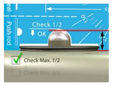
If the gauge lies flat on the actuator and there is no interference with the push rod, the check has passed and you should move on to test for minimum permitted height.
