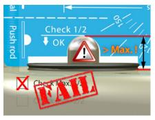
If the gauge does not lie flat on the actuator due to interference with the push rod the check has failed.
