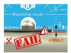
The height of the seal should not drop below 3 mm. If the seal height is lower than the line marked "min. thickness check 1/1", the check has failed.
