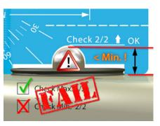
If the push rod height is lower than the "OK" line, the check has failed.
